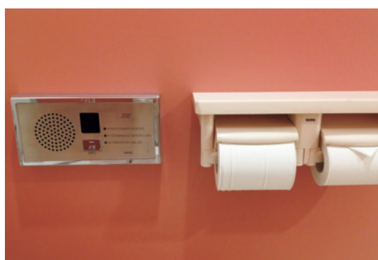
Figure 1 An example of a device called the ' Sound Princess ' (1) in a university toilet. When a hand is placed over the sensor, the sound of flushing water will be played for 25 seconds. If the switch below the sensor is pressed the sound will become quieter and then stop.
